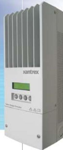
The Xantrex XW Solar Charge Controller (XW SCC) is a photovoltaic (PV) charge controller that tracks the electrical maximum power point of a PV array to deliver the maximum available current for charging batteries. When charging, the XW SCC regulates battery voltage and output current based on the amount of energy available from the PV array and state-of-charge of the battery.
